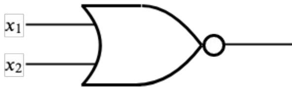
$$f = x_1 \downarrow x_2 = \overline{x_1 + x_2} = \overline{x_1} \overline{x_2}$$
