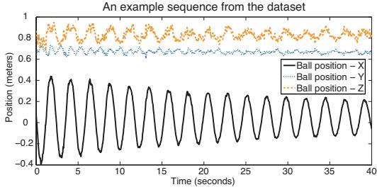
**Fig. 5** One of the 20 sequences of the real pendulum trajectory as recorded by our system and used as dataset for the experiments. The first three oscillations were used to make the filter converge before driving actual arm movements
