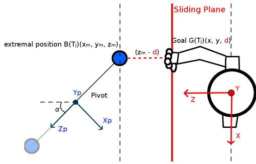
**Fig. 1** Top view of the reaching task performed by the robot. At each oscillation the iCub moves its right hand to the position  $G(T_j) = (X_m, Y_m, d)$ , where  $B(T_j) = (X_m, Y_m, Z_m)$  is the position of the target at the minimum distance ( $Z_m - d$ ) during the oscillation
