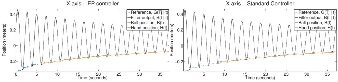
**Fig. 8** Behaviour of the two algorithms during an oscillation sequence. The EP controller has  $\text{Th} = 4 \text{ mm}$ . Results on the X axis are shown
