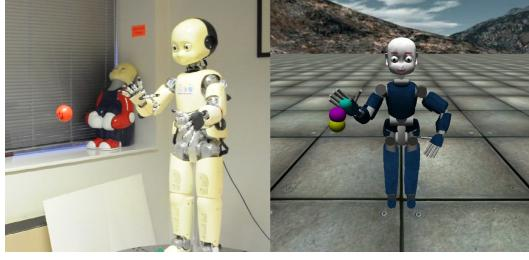
**Fig. 4** Left: The iCub humanoid robot tracking the oscillating target (red ball). Right: the iCub Simulator during the test. The blue ball is the predicted goal position, the yellow ball is the output of the 3D tracker and the purple ball is the output of the filter
