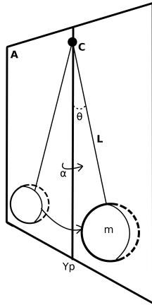
**Fig. 2** Pendulum model. 2D pendulum oscillating on a plane  $A$  rotated of an angle  $\alpha$  on the  $Y_p$  axis
